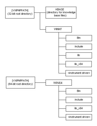
Each instrument has a directory under the framework subdirectory. For example, a Tektronix VX4385 will be found in the directory TKVX4385, which is the name of the instrument driver.
