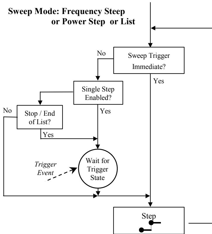
from start to stop with fixed increments (steps) or from a list of arbitrary values. The duration of one step is defined with Dwell Time. Setting the Sweep Trigger attribute to External or Software Trigger will delay the start of the next step until the specified trigger event occurs.
