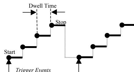
Single Step and Trigger External / Software:
