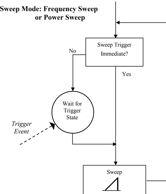
Setting the Sweep Trigger attribute to Immediate will continuously generate sweeps (either frequency or power sweeps). The duration of one sweep from start to stop is defined with Frequency Sweep Time or Power Sweep Time. Setting the Sweep Trigger attribute to External or Software Trigger will delay the start of the next sweep until the specified trigger event occurs.
