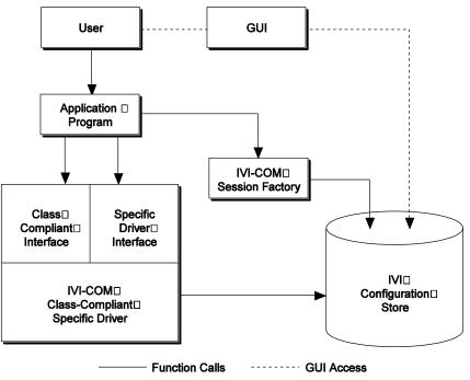
Figure 2-4. Using an IVI-COM Class Compliant Specific Driver
