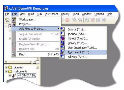
Note: Any of the three files listed above will work. Adding one of the HP 34401A instrument driver files loads that instrument driver. View the available functions in the library tree in the workspace window.
