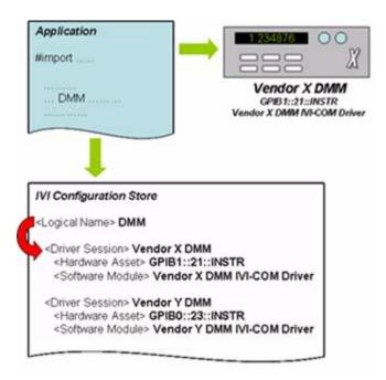
In the illustration below, we replace the Vendor X DMM with a Vendor Y DMM. All we need to do is change the LogicalName so that it points to a different DriverSession. In this example, change the LogicalName so that it point to the Vendor Y DriverSession. We do not need to make any modifications to the application itself. All changes are contained within the Configuration Store.
